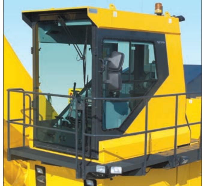
OPG top guard level 2 integrated into the cab
