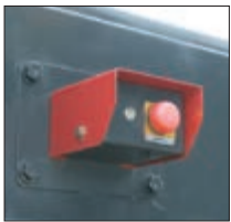
Emergency stop switch (with engine start lock function)
