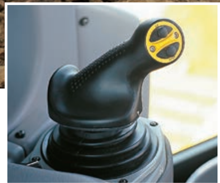
Palm Command Control System (PCCS)
