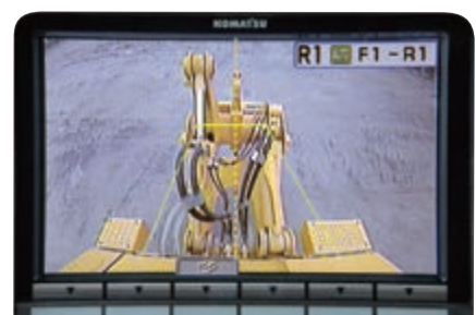
Fully integrated rear-view camera system
